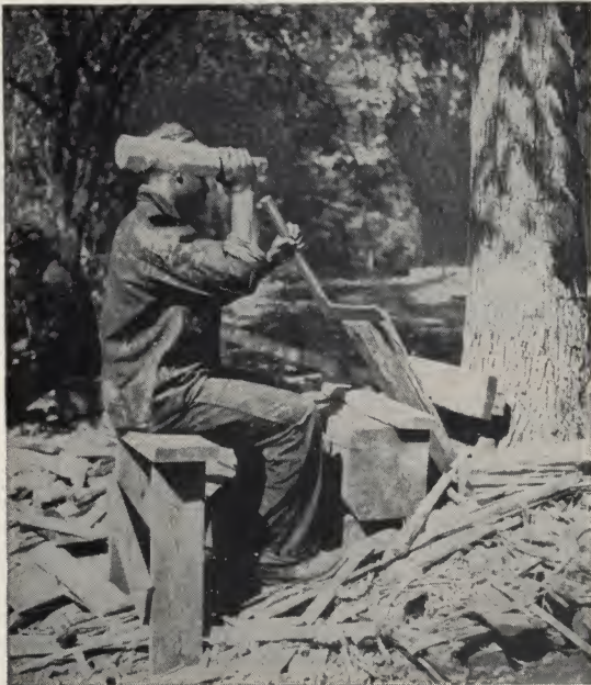
FIGURE 20.—Splitting shakes with the froe.
